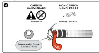
NOTE: Do NOT apply grease if the remote lever is to be installed on carbon handlebars.
